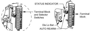
Activate/De-activate Silent Arming (No 3-Beeps): Remove all power and open the door/ door contacts. Turn key fully CW to disarm the unit. Hold the Call Bell button (terminals 7&8) closed and apply power. Use a jumper wire if the Call Bell feature is not used. Red and Green LED's flash and siren chirps twice, after approximately 5 seconds release the Call Bell or remove jumper and install unit per instructions.
